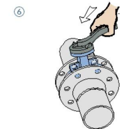
⑥ 待焊口冷却后再安装蝶阀，保证蝶阀在法兰中有足够的活动空间，以防止蝶阀被损坏。并保证阀板有一定的开度 When the flange is cooled to normal temperature, Then install butterfly valve, Ensure the butterfly valve has enough space in two flanges, Prevent that damage the butterfly valve, Ensure disc has some open angles
