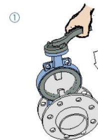
① 将蝶阀放置于预安装的两片法兰间 Put the butterfly valve into between preinstall two flanges
